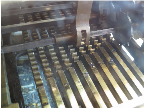
Figure 5. Setting a digit of the multiplicand
