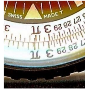
Tick mark at 30 out of alignment. 30 on the inner scale aligns with 29.8 on the outer scale
