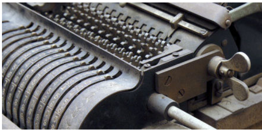
Figure 6.2 - Thompson's difference engine, the transfer mechanism
