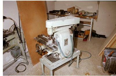
Figure 10: Mechanically fed Router cuts the Central Keyways
