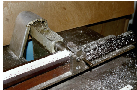
Figure 14: Chamfering Ends of Slides
